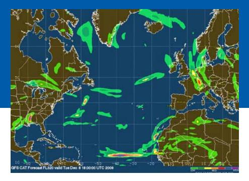
Using state-of-the-art algorithms, ENSCO produces automated clear air turbulence (CAT) forecasts that cover the entire globe. These products, which are specially tailored for international flight operations, forecast CAT at 10 flight levels between FL240 and FL440. Each flight level package contains forecast snapshots valid every 3 hours for the next 30 hours. They are updated automatically every 6 hours using high-resolution model output from the National Weather Service.
