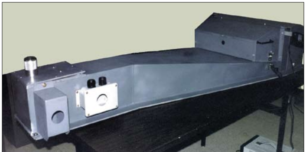
The Automated Air Hose Inspection system detects low-hanging or damaged air hoses and notifies appropriate railroad personnel.
