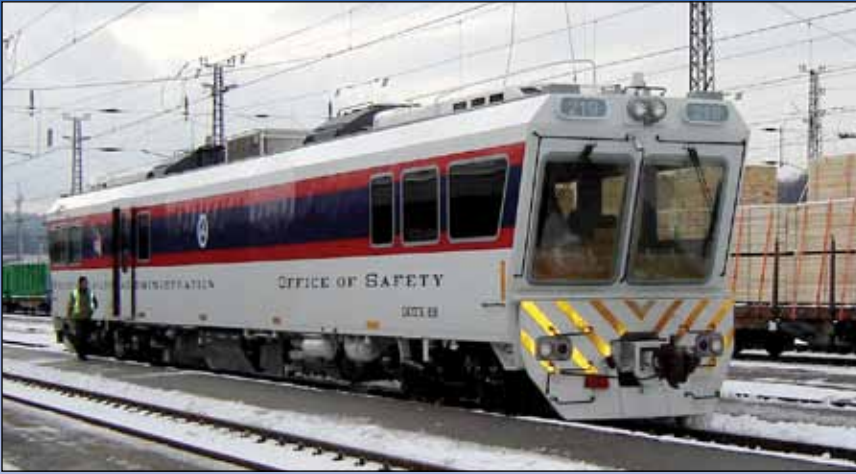
FRA's DOTX 219 Track Geometry Measurement Vehicle.
