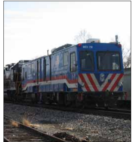
Federal Railroad Administration's (FRA) DOTX 218 Deployable Gage Restraint Measurement Vehicle.
