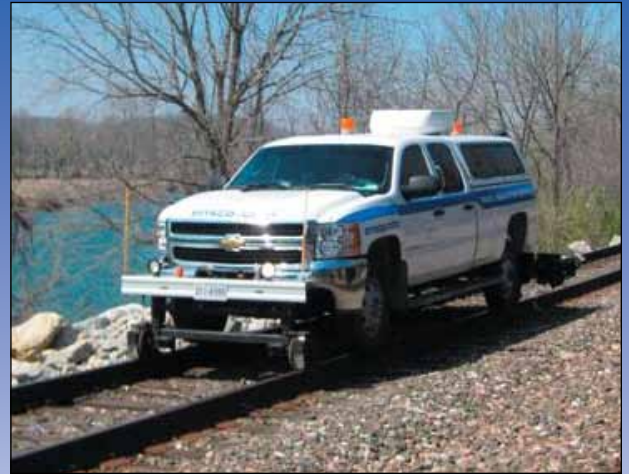
ENSCO equipped Hi-Rail inspection truck.
