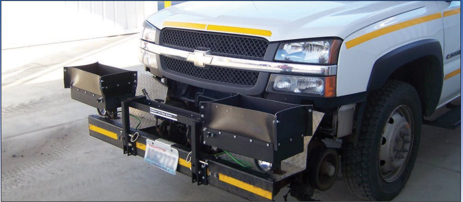
Removable hi-rail bumper mount system designed for secure storage and road travel.
