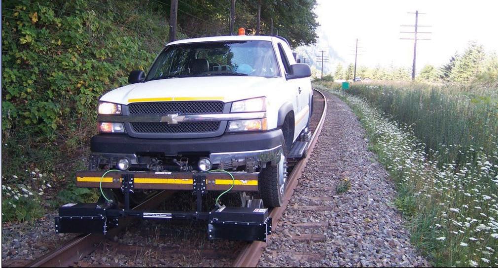
RailScan offers continuous gage and crosslevel measurement up to 35 mph.
