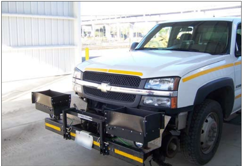
Removable Hi-Rail bumper mount system designed for secure storage and road travel.
