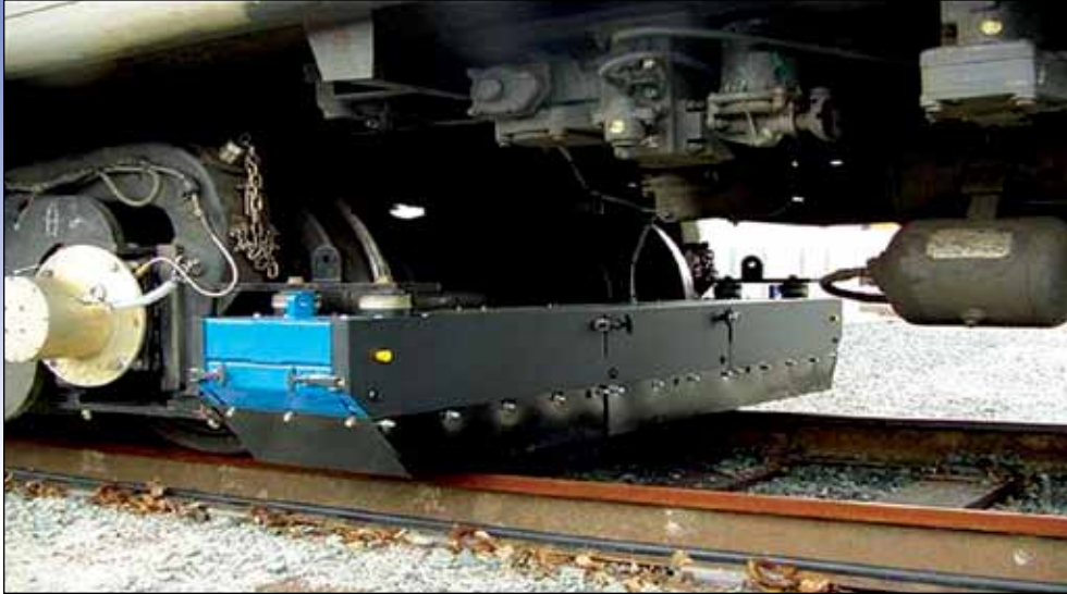
Track Geometry Measurement System
