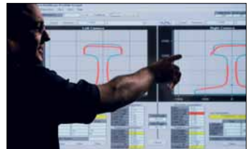
ENSCO's Rail Profile Measurement Service provides critical information for rail grinding and replacement programs.
