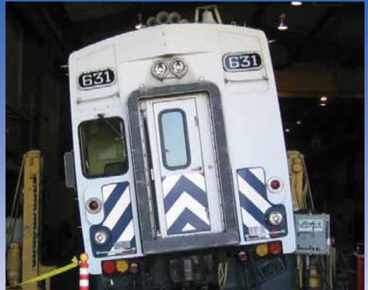
Wheel unloading test being conducted.
