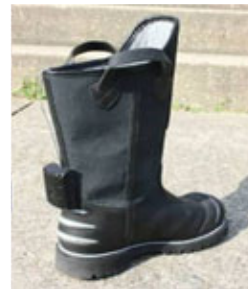
Figure 13: IMU mounted on heel of firefighter's boot.
