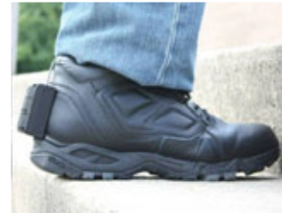
Figure 4: MEMSense nIMU mounted on operator's boot.
