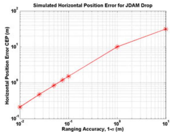
Figure 4: Position errors upon impact of a JDAM based solely on the integration of a HG1900 IMU and range measurements after the bomb drop.
