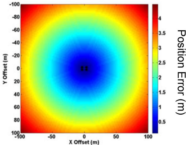
**Figure 6: Approximate horizontal position error plot for four antennae mounted on corners of troop carrier.**
