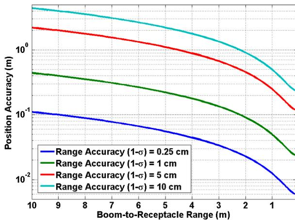
**Figure 8: 3D position accuracy for a single suite of range measurements that were simultaneously measuring to a radio located on the fuel receptacle of the vehicle being refueled. The position errors are based on a simple PDOP calculation given the three radio locations (two mounted on the tips of the steering vanes and one co-located with the tip of the refueling boom) and expected ranging accuracies.**
