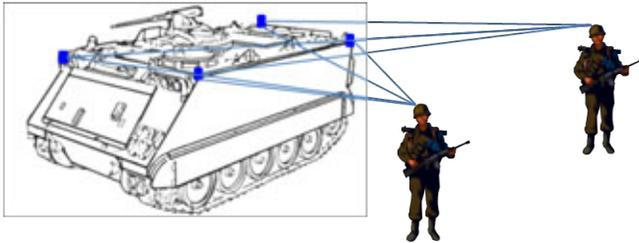
**Figure 5: Dismounted soldier concept for integration of RF range measurements from a single ranging radio mounted on top of the troop carrier.**
