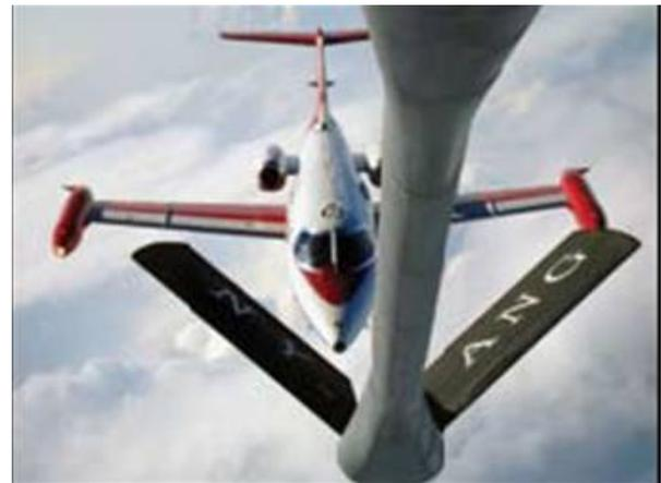
**Figure 7: A flying boom approaches a Learjet that is being flown as a surrogate for a UAV during a demonstration of automated aerial refueling.**
