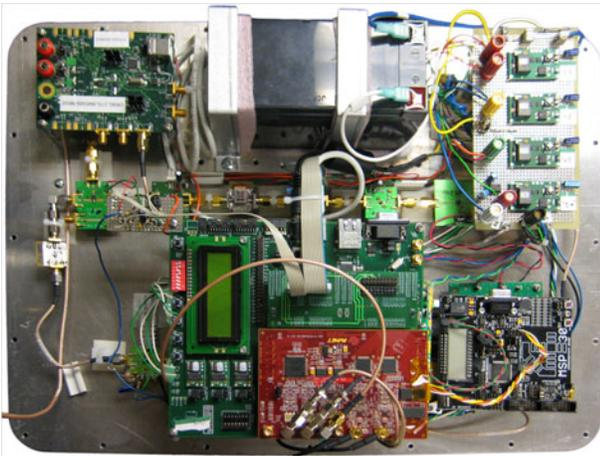
**Figure 1: Prototype ranging radio platform.**
