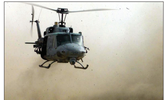
DVE solution delivers increased situational awareness to pilots, during brownout conditions generated by rotorcraft downwash. Photo credit: U.S. Navy, Naval Air Systems Command
